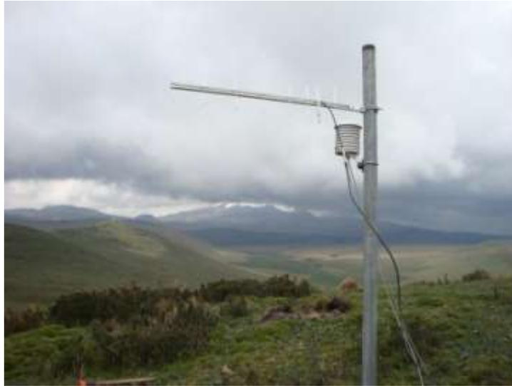
**Figura 2.47** Antena Yagi
